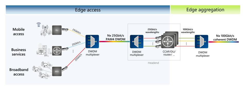
25Gbit/s DWDM links with up to 40km reach from any device with an SFP28 port
